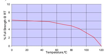
Polypropylene to Steel treated with  ${\bf START\text{-}UP\ PROMOTER\ SU\text{-}P42}\ \&\ {\it bond\ with\ ethyl\ instant\ adhesive}$
